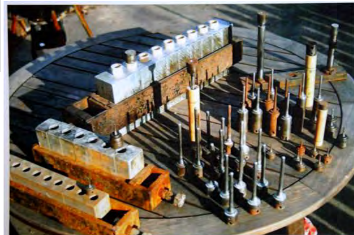
This equipment is for the manufacture of handmade black powder rocket motors. The long mandrels are for making high thrust, short duration motors to lift heavier loads. The short mandrels with the narrow thrust diameters are for making long duration, end-grain burning motors capable of sending rockets with light payloads to higher altitudes. Multi-staging is also common.
