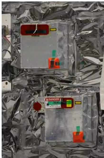
A close-up of the two TriDAR rendezvous and docking laser systems which provide automated, real-time visual guidance for navigation, rendezvous and docking.
