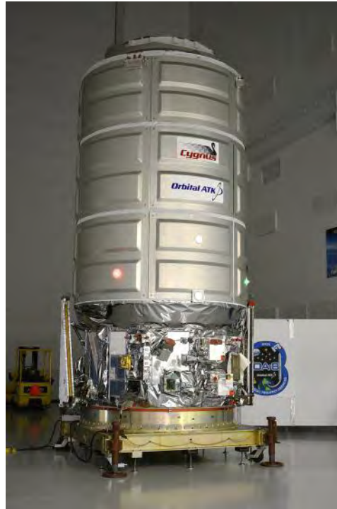
The Cygnus spacecraft was mounted vertically on a platform with its two solar arrays in their retracted position. The OA-8 mission patch is seen to the left.
