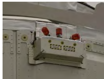
Close up of some of the many thrusters attached to the Cygnus cargo module.
