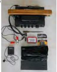
wireless system into a single 'crib notes' sheet that guides the operator through the whole system assembly and start-up procedure. These guidelines include the correct order to connect the 12 volt battery, the correct order for the activation of the wireless and amplifier systems, the speakers' wire connections and the volume and tone settings. Both the corded microphone and the wireless microphone have been tested and both work with
