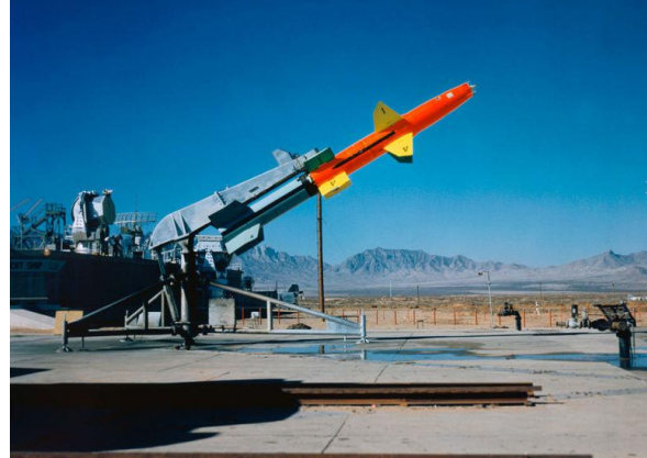
The '60s Talos surface to air missile was an early ramjet design.
