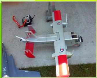
Brother Toshi's new ship. She's a VTOL! The wing articulates and the motor on the rear fuselage gives lift.
