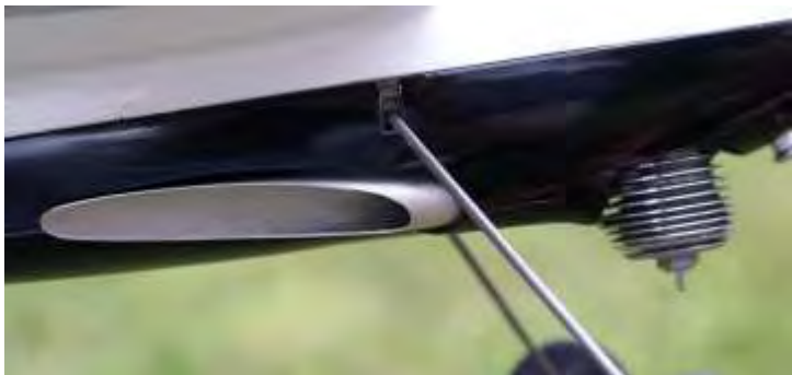
Slash-cut pipe on Al Ferraro's Fora 15 entry.
