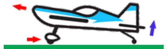
No problem. Just maintain full up elevator, right? As the plane gains speed, the forces on the elevator will increase the downward pressure on the tail wheel to maintain good steering authority. True, but to a point. Remember that high angle of attack on the wings. You could end up with flying with full elevator, low airspeed, a high angle of attack, and no rudder authority. Uh oh.
