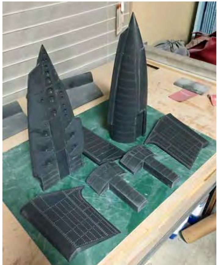
Detailed plug parts ready for molding.
