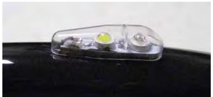
**Finished wingtip unit. Clear lens held in place with a thin application of clear silicone.**
