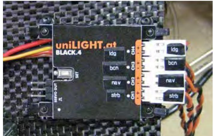
**Controller installed on equipment tray. Identification tags placed on unit and attaching plugs for easy reference.**
