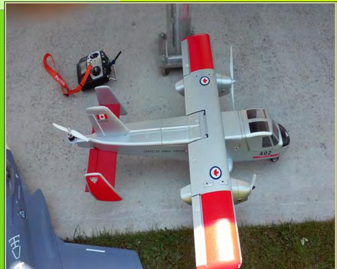
Brother Toshi's new ship. She's a VTOL! The wing articulates and the motor on the rear fuselage gives lift.
