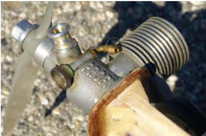
**Why give yourself a migraine trying to use a TD 049 in 1/2A Proto? Combat engines like this Profi or the Cyclon and Fora are so much easier to deal with. The needle assembly is designed to work with a bladder system, so you may need to install a different assembly if using suction. APC props are plenty good to get started.**
