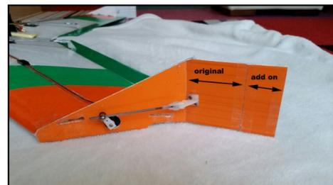
I have now increased the rudder size to about 10 square inches from the original 6. My maximum deflection is 50 degrees. I have moved Gear control to a 3 position switch which allows two different levels of braking.
