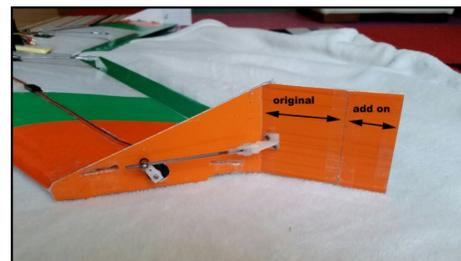
I have now increased the rudder size to about 10 square inches from the original 6. My maximum deflection is 50 degrees. I have moved Gear control to a 3 position switch which allows two different levels of braking.
